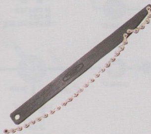
COG REMOVER Model: TA-131 (Code No.58129951) For 1/2" x 3/32" chain Model: TA-130 (Code No.58129950) For 1/2" x 1/8" chain Specifications ● Material: Steel ● Use: Freewheel & cassette cog (Model: TA-131) Track cog (Model: TA-130)
