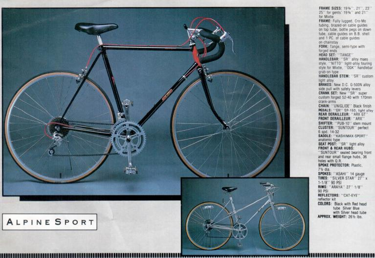
RIMS: "ARAYA" 27" 1/8" 90 PSI PSI "CAT-EYE" reflector kit COLORS: Black with Red head tube Silver Blue with Silver head tube APPROX. WEIGHT: 26 ½ lbs. REAR DERAILLEUR: New
