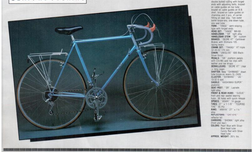
FRAME SIZES: 19", 21", FRAME: Fully lugged. Cro-Mo double butted tubing with forged ends with adjusting botts, brazed-on cable guides on top tube brazed on cable guides on B.B. shell, brazed-on cable guides on chainstay and 2 pcs. of carrier fitting on seat stay. Two water bottle braze-ons, one down tube, one seat tube bottle braze-ons, one down tube, one seat tube
